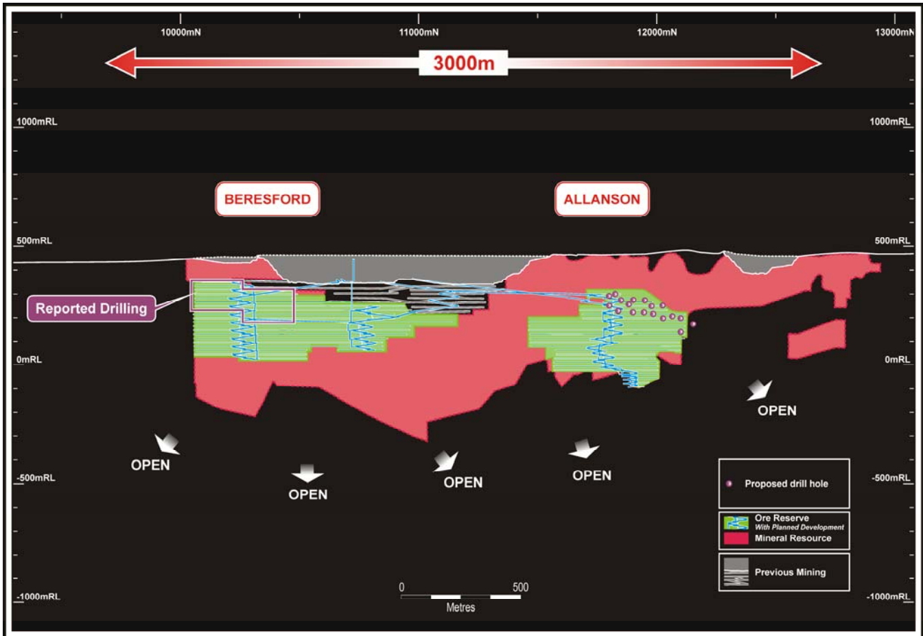
Figure 1: Longitudinal section of the Westralia Deposit showing the location of the Beresford Ore Reserve with planned development and the recently completed 24 hole, 5,730m in-fill diamond drilling program reported in this announcement (purple box). Also shown is the 18-hole in-fill program currently underway targeting the Allanson Underground Ore Reserve (purple dots).
