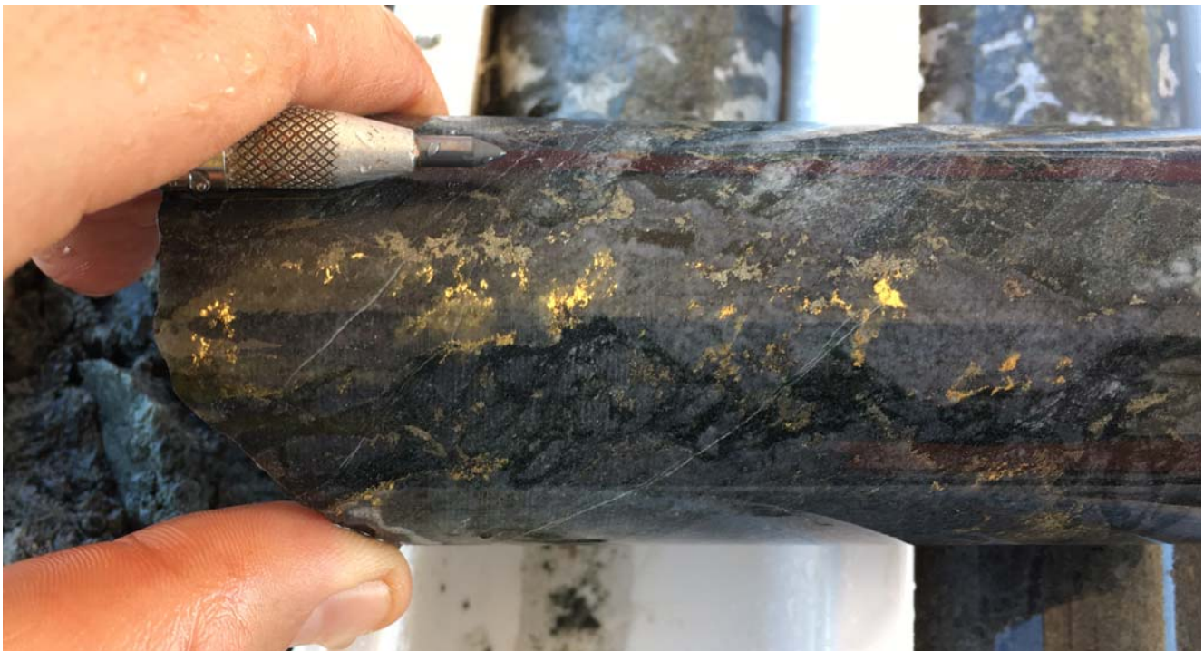
Figure 2: Coarse visible gold from the Contact BIF in drill hole 17MMDD0335 returned 7.0m @ 31g/t Au including 1.5m @ 135.2g/t Au. Core width is 50mm. The intersection is from outside the current Ore Reserve at Beresford and provides a possible additional early production source once mining commences in the second half of CY2017.
