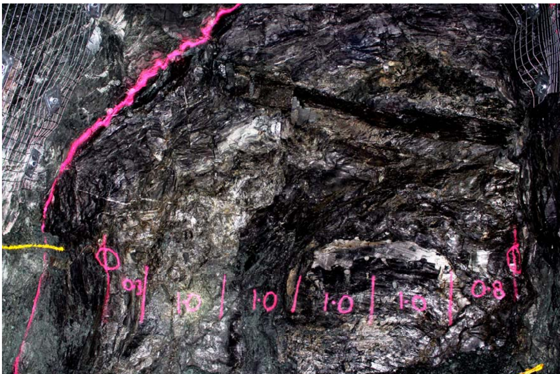
Figure 1 – First ore intersected at the 2297 access, Beresford underground gold mine. Note the highly sulphidised BIF host to the gold mineralisation (bronze/brown colour). The painted pink line on left hand side of photograph is the hangingwall contact of a highly competent basalt unit.
