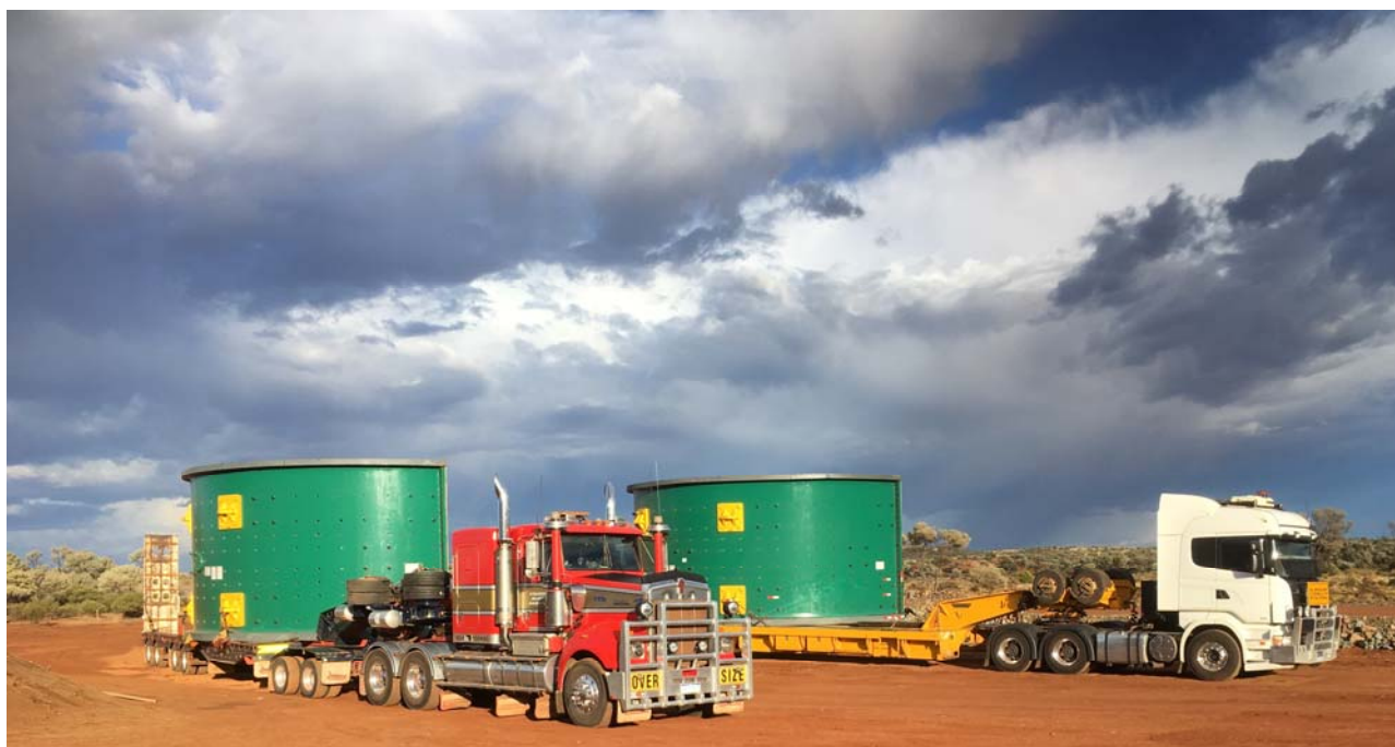
Figure 1 – Arrival of the two halves of the 8.5m diameter, 3.5m long SAG mill to the Mt Morgans site.
